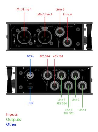
The audio connectors are on the sides of the unit; analogue inputs are on the left, while analogue outputs and all digital I/O are on the right side. Connections of a similar function are grouped together, with the low channel numbers within each group towards the rear of the unit.
